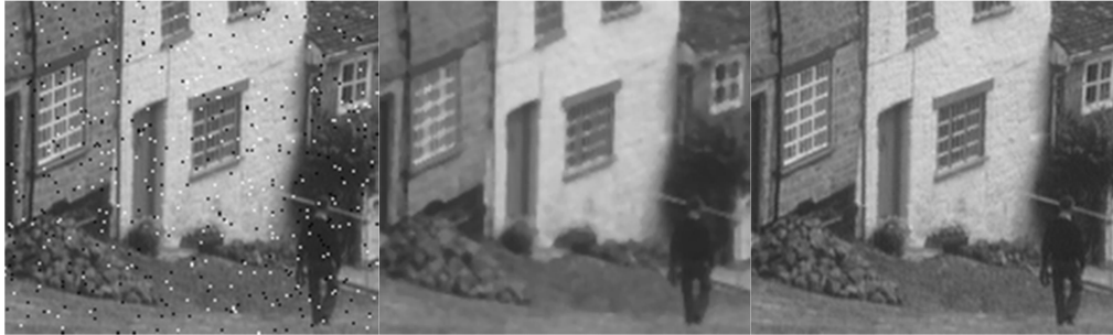
Figure 2. From left to right: a. Salt and pepper noise; b. median filtered image; c. image filtered with our method
