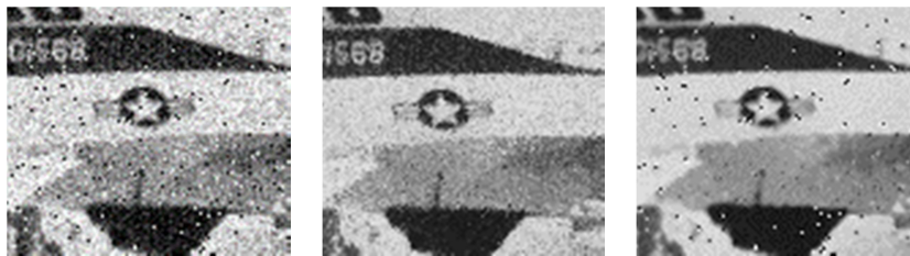
Figure 5. From left to right: a. Image affected by salt and pepper and Gaussian noise; b. Image filtered without salt and pepper noise filter; c. Image filtered using OpenCV FNLMD
